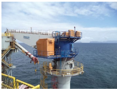
Shrink wrap covers as many rig surfaces as possible to prevent corrosion during stacking.
