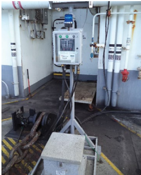
Remote Bilge Monitors are powered by generators with backup power from solar panels as long as rigs remain stacked.
