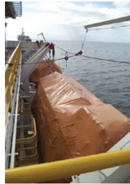
Shrink wrap covers as many rig surfaces as possible to prevent corrosion during stacking.
