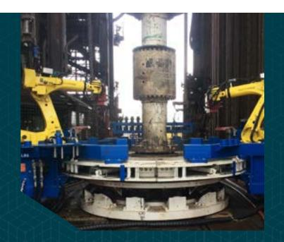
risks. Thus, we teamed up with Offshore Robotics and ARC Specialties to come up with a solution to remove personnel from the drill floor during riser operations and conduct these operations more efficiently. ARC Specialties and Offshore Robotics brought vast knowledge and experience with automation in a variety of industries, and Transocean contributed industry-leading offshore drilling operations expertise to the project. The outcome: A Robotic Riser System.
